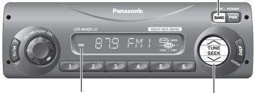
FM stereo indicator, lights while receiving an FM stereo signal.
